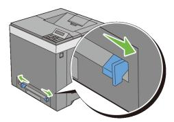
2 Hold both sides of the print media facing down close to the single sheet feeder, and push it 8 cm to 9 cm (4 inches) into the printer until it automatically feeds.
